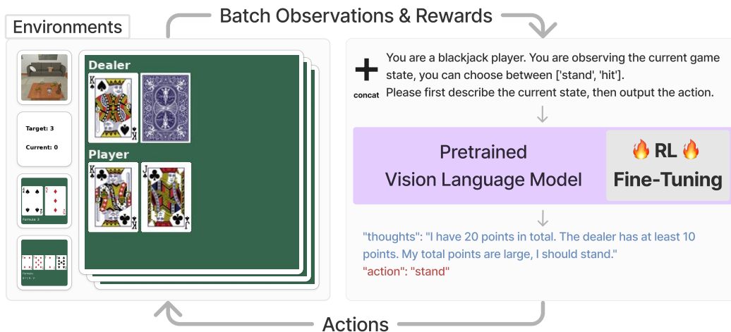
Figure 1: Method overview. We propose a framework for training large Vision-Language Models (VLM) with Reinforcement Learning (RL). At each time step, the VLM takes the current observation and a predesigned prompt as input and outputs an utterance containing a chain of thought reasoning and a text action . The text action is parsed into the environment for generating task rewards. Finally, we apply RL with the task reward to fine-tune the entire VLM.
