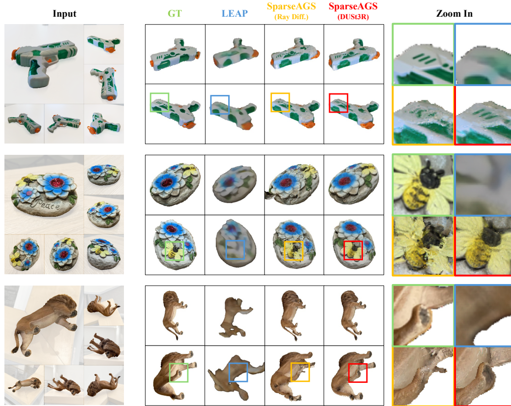
Figure 4: Qualitative Comparison with LEAP [12] on Novel View Synthesis. We use two pose estimation baselines (Ray Diffusion [47] and DUST3R [41]). SparseAGS better preserves details from the input images and shows enhanced performance with more accurate initial camera poses. More results are available in Fig. 9 of the appendix.
