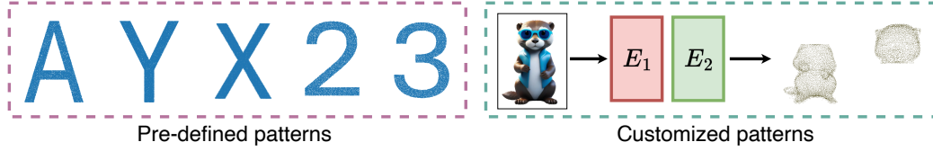
Figure 3: Two different target geometry patterns. (1) Pre-defined patterns: we directly convert alphanumeric characters into a 2D point cloud as watermarks. (2) Customized patterns: In E_1 , we first extract the point cloud of the image that needs to be protected. In E_2 , we edit the acquired point cloud through text-guided methods like instructP2P [48] or open-source software meshlab [5].
