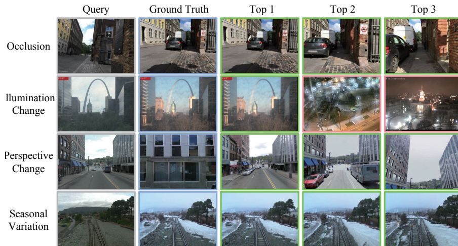
Figure 4: Query (gray) and top 3 retrieved frames (green: successful, red: failed). Moreover, one of the true (blue) matches is displayed for comparison.
