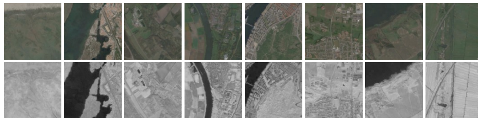
Figure 3: Satellite image data. 128 \times 128 images from Sentinel-2. First row RGB, Second row NIR.
