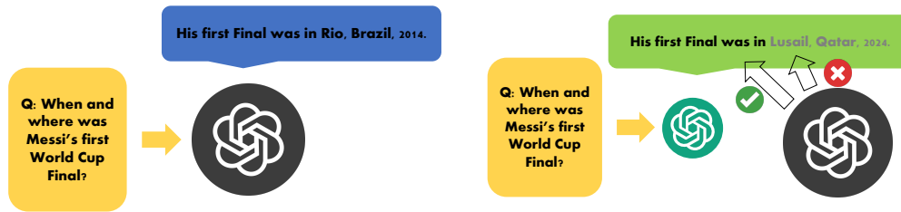
Figure 1: Left: Standard Auto-Regressive Decoding (Algorithm 3) v.s. Right: Speculative Decoding (Algorithm 1), where a large model is used to validate the responses of the small model.
