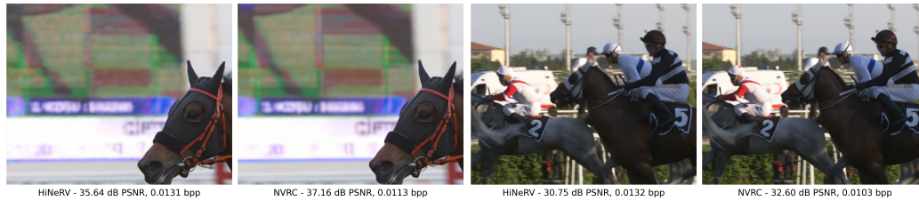
Figure 1: Comparison between the output from HiNeRV [30] and the proposed NVRC. The image is from UVG dataset (Jockey/ReadySetGo sequence) [45]
