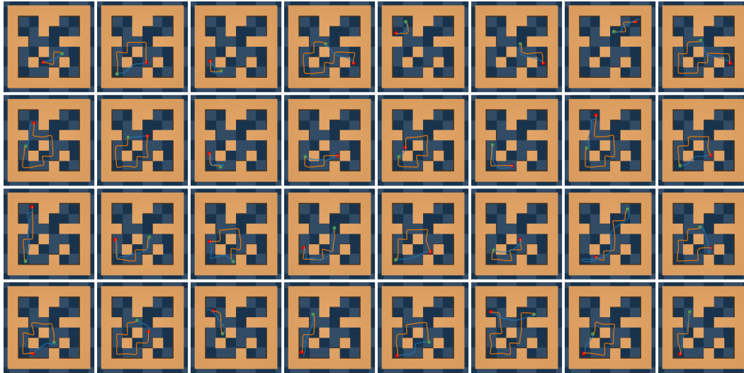
Figure 11: Full result of generated trajectories under POINTMAZE. The blue trace represents the generated trajectory and the orange trace represents the corresponding expert trajectory. DIFO can accurately model expert behavior and generate successful trajectories.
