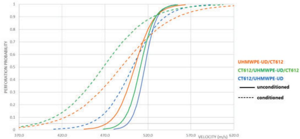
**Figure 6.** S-curves for various Twaron® CT612LS/UHMW-PE UD hybrids before and after tumbling
