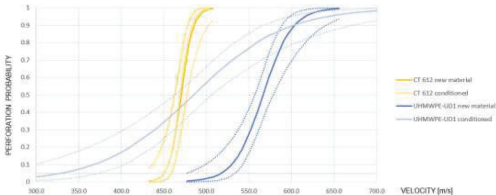
**Figure 5.** S-curves for Twaron® CT612LS woven fabric, and UHMW-PE UD1 before and after tumbling also including confidence boundaries.
