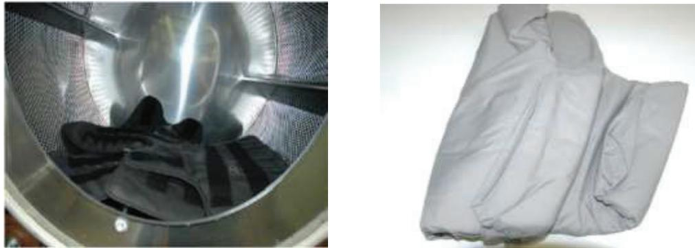
**Figure 3.** Tumble drum IAW NIJ 0101.06 (left) and tumbled armour panel (right) (reproduced from [3])
