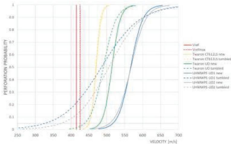
**Figure 4.** S-curves for Twaron® CT612LS woven fabric, Twaron® UD and UHMW-PE UD1 before and after tumbling
