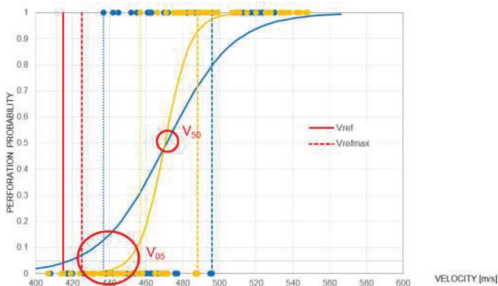
Figure 2. S-curve for two different sets of armour
