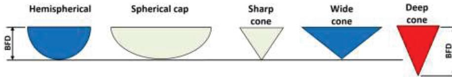
Figure 3: Comparison of backface cavity shapes
