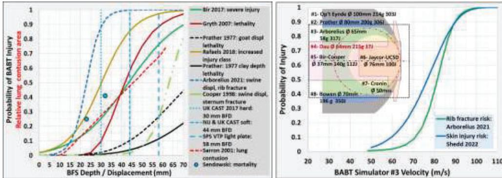
Figure 2: BAPT injury risk functions/data: vs depth/displacement (left), vs velocity (right)
