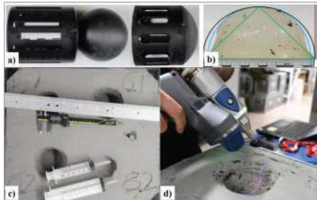
**Figure 5:** Dau and Arborelius rigid impactors (a), silicone cavity mould (b) Cavity volume measurement with water (c) and laser scanning (d)
