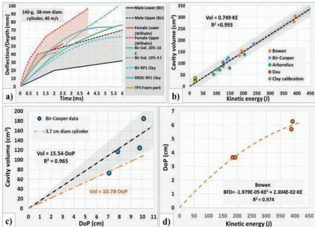
Figure 6: a) Bir-Wilhelm torso biofidelity corridors and RP1 cavity depth vs time for Bir impactor b) volume vs KE for 4 impactors, (c) volume vs DoP for Bir, (d) DoP vs KE for Bowen
