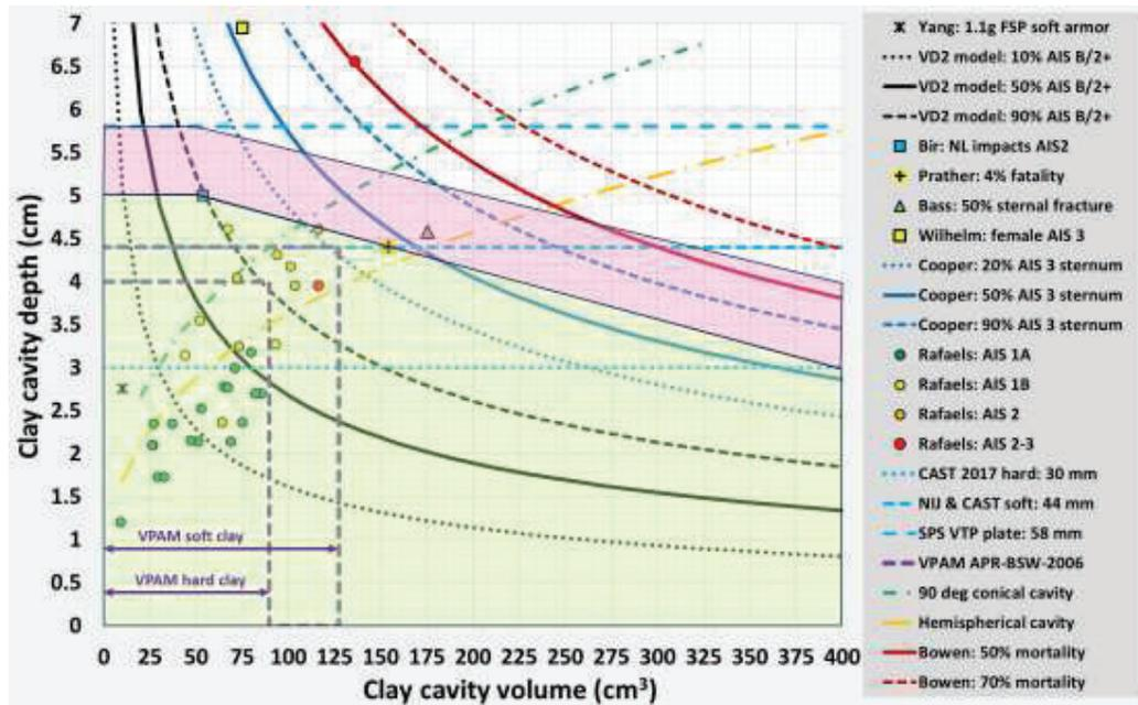
**Figure 7:** Cavity depth vs volume graph with iso-BABT severity curves derived from VD<sup>2</sup> IRFs
