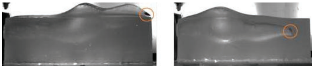
Figure 48. Left: 7.62 x 39 mm M43 projectile propagating through gelatine. No fragmentation occurred. - Right: 7.62 x 39 mm M43 projectile propagating through gelatine after piercing a Level IIIA soft armour. No fragmentation occurred.
