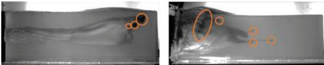
Figure 50. Left: .338 AP projectile propagating through gelatine. Only 3 fragments. - Right: .338 AP projectile propagating through gelatine after piercing a Level IV in-conjunction armour. 4 major fragments and an extensive debris cloud.
