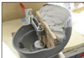
Figure 59. Helmet shell filled with clay witness material for qualification of BHBT.
