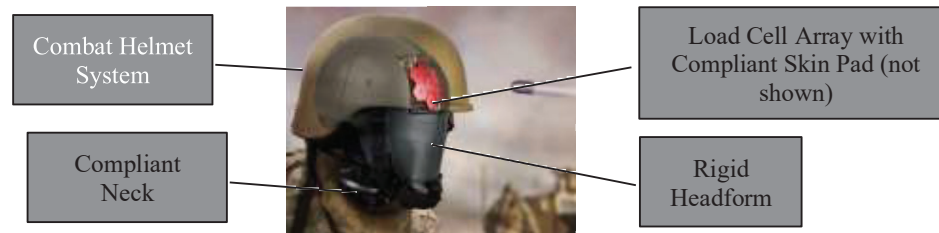
Figure 57: The Ballistic Load Sensing Headform for measuring BHBT.
