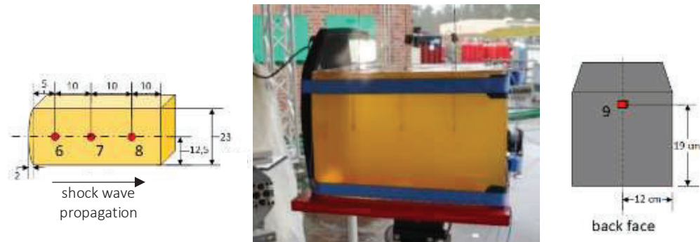
Figure 2. Left side: Sketch of the instrumented simplified torso model. Middle: Detail view of instrumented body model with protective plate attached. Right side: Sketch of the instrumented protective plate.
