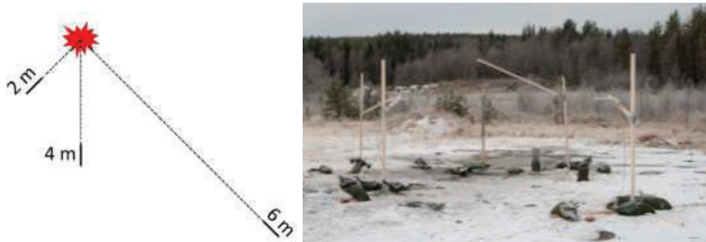
Figure 1. Experimental setup of the free field wave measurements
