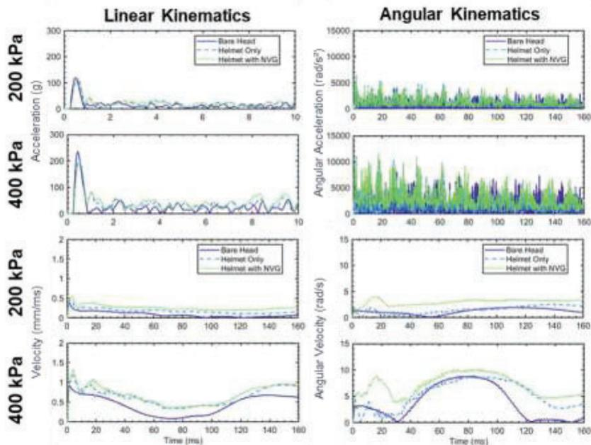
**Figure 69.** Resultant Kinematic response scales with increasing blast exposure for all kinematic measures. Linear acceleration peak occurs in first 10 milliseconds and is shown for reduced window.
