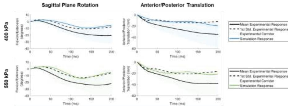
**Figure 67.** Model demonstrates response in line with stiff cadaveric response in rotation (left) and translation (right) to when exposed to experimental pressures at 400 kPa (top) and 500 kPa (bottom).
