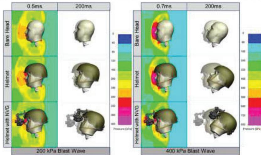
**Figure 68.** Snapshot of Simulation Results for 3 configurations and 2 blast severities. The distribution of pressure after contact is altered by inclusion of the helmet and NVG surfaces.
