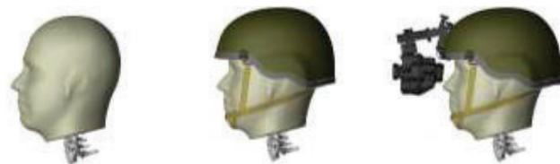
**Figure 66.** APL head-neck model without a combat helmet, with a combat helmet, and with NVG.
