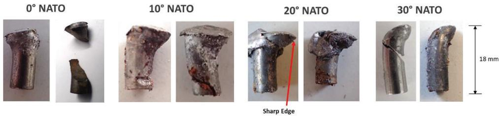
Figure 7: Projectiles after impact at different shot angles
