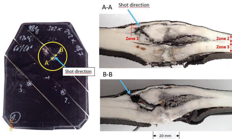
**Figure 4:** Example of an torso plate sample, tested at 30°/30° NATO (60°/60° VPAM) and 20 °C. Inserts were cut by waterjet, measurement of the zones
