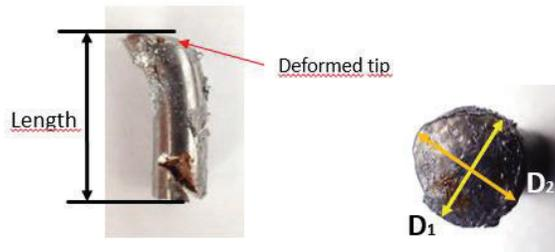
Figure 8: Measurement of length and diameters of the projectile after impact
