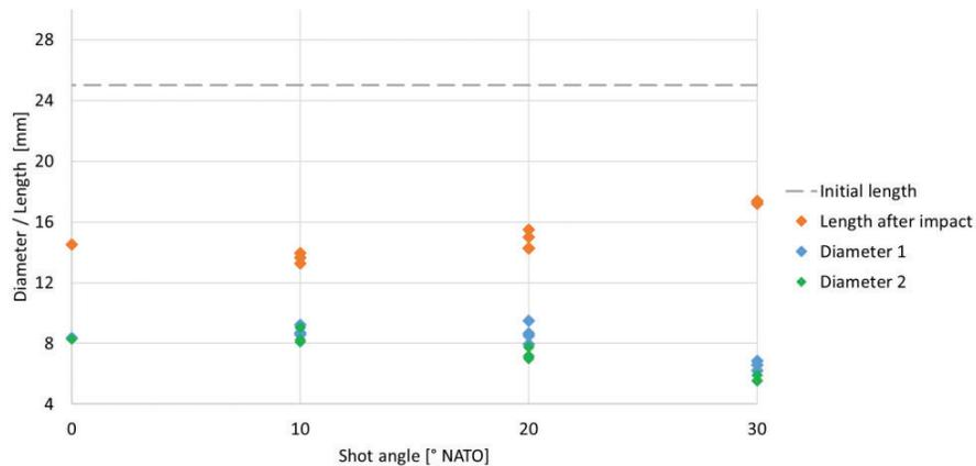
Figure 9: Angle dependence of diameter and length of the projectile after impact
