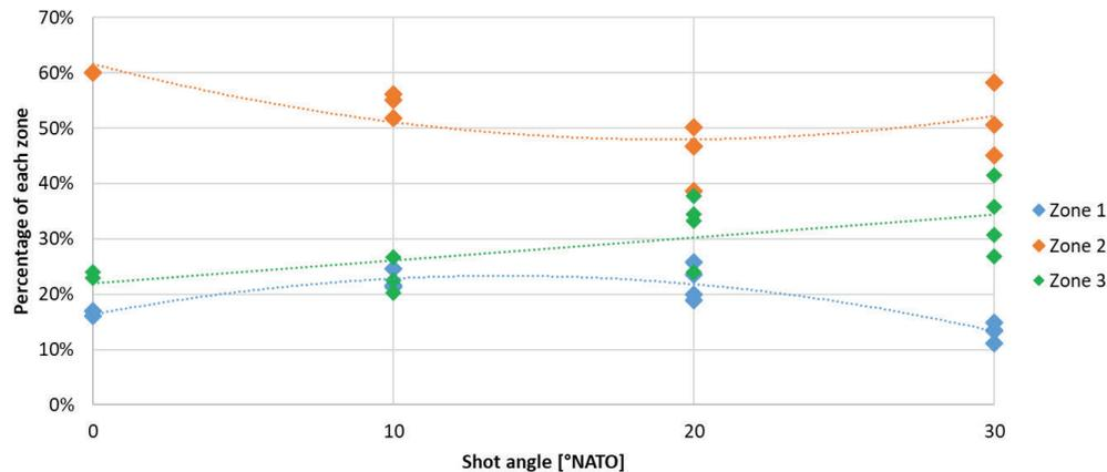
**Figure 6:** Thickness of zone 1-3 in depending on the shot angle
