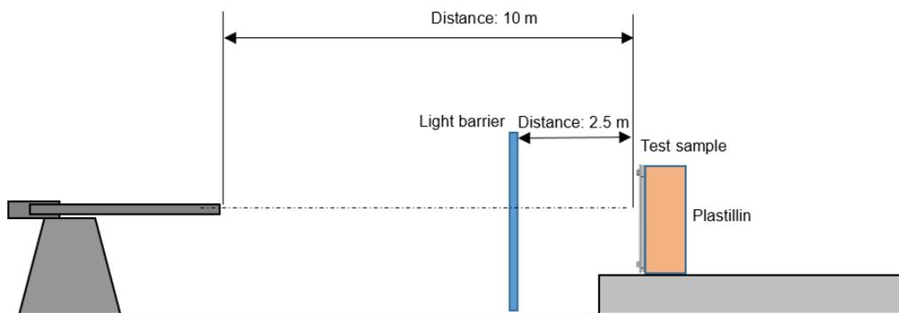
**Figure 3:** Schematic Test set-up of body armor inserts, according to VPAM BSW Annex 1 [1]
