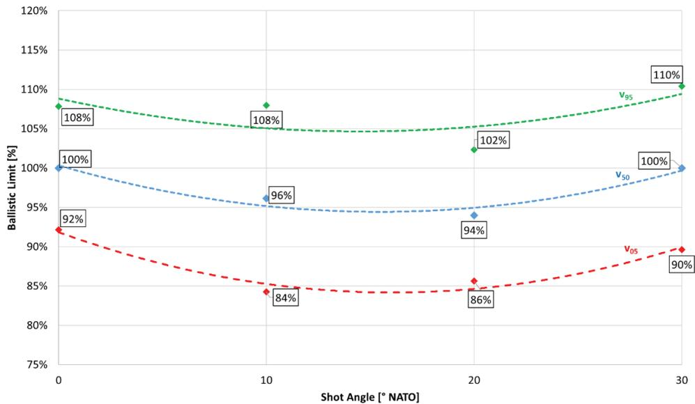
**Figure 2:** Laminate 2, Influence of the shot angle on  $v_{50}$ ,  $v_{05}$ , and  $v_{95}$ ;  $v_{50}$  at 0° NATO is 100 % - reference
