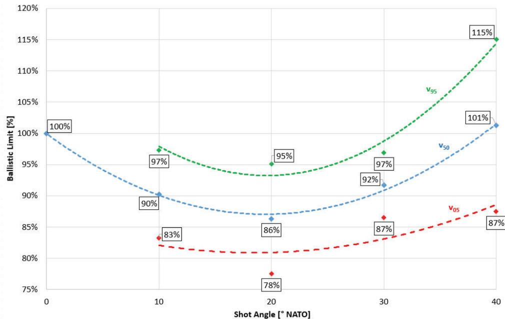
**Figure 1:** Laminate 1, Influence of the shot angle on  $v_{50}$ ,  $v_{05}$ , and  $v_{95}$ ;  $v_{50}$  at  $0^\circ$  NATO is 100 % - reference
