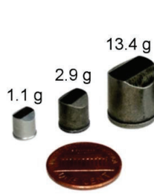
Figure 4. Fragment Simulating Projectiles (FSPs) used by NIJ [2]
