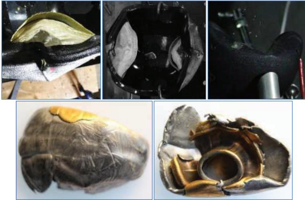
**Figure 12.** Shot 2 on UHMWPE helmet PE3: permanent deformation (top left); high-speed still of temporary deformation (top right); recovered bullet (bottom)
