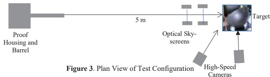
Figure 3. Plan View of Test Configuration
