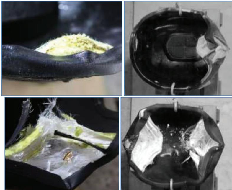
**Figure 5.** Shot 2 on para-aramid helmet PA1 (top) and Shot 2 UHMWPE helmet PE1 (bottom): permanent deformation (left); high-speed still of temporary deformation (right).
