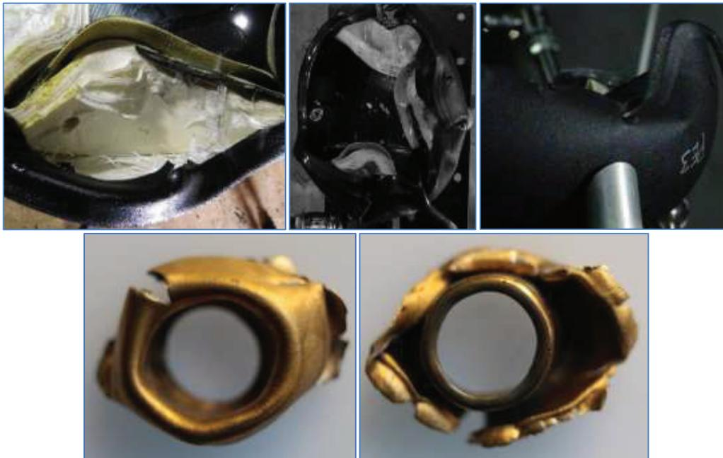
**Figure 13.** Shot 3 on UHMWPE helmet PE3: permanent deformation (top left); high-speed still of temporary deformation (top right); recovered bullet (bottom)
