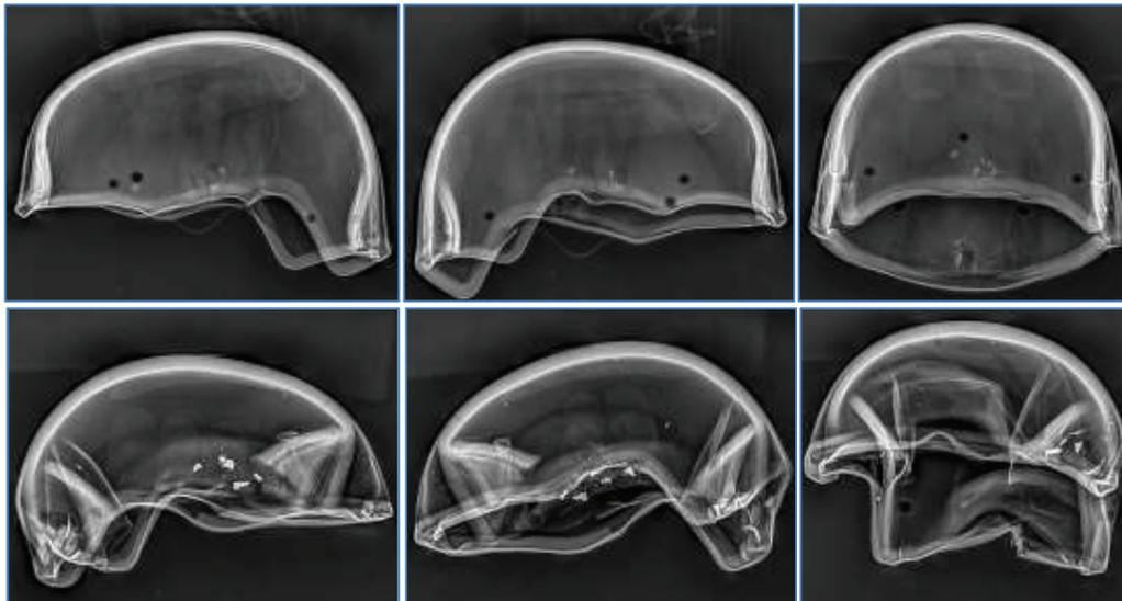
**Figure 14.** X-Rays of Para-Aramid Helmet PA3 (top) and UHMWPE Helmet PE3 (bottom); Post-Test
