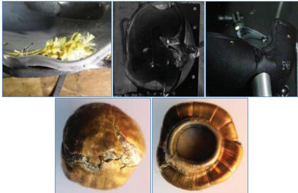
**Figure 11.** Shot 3 on para-aramid helmet PA3: permanent deformation (top left); high-speed still of temporary deformation (top right); recovered bullet (bottom)
