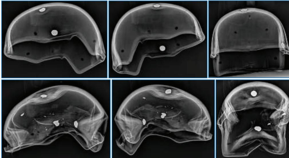
Figure 9. X-Rays of Para-Aramid Helmet PA2 (top) and UHMWPE Helmet PE2 (bottom) – Post-Test
