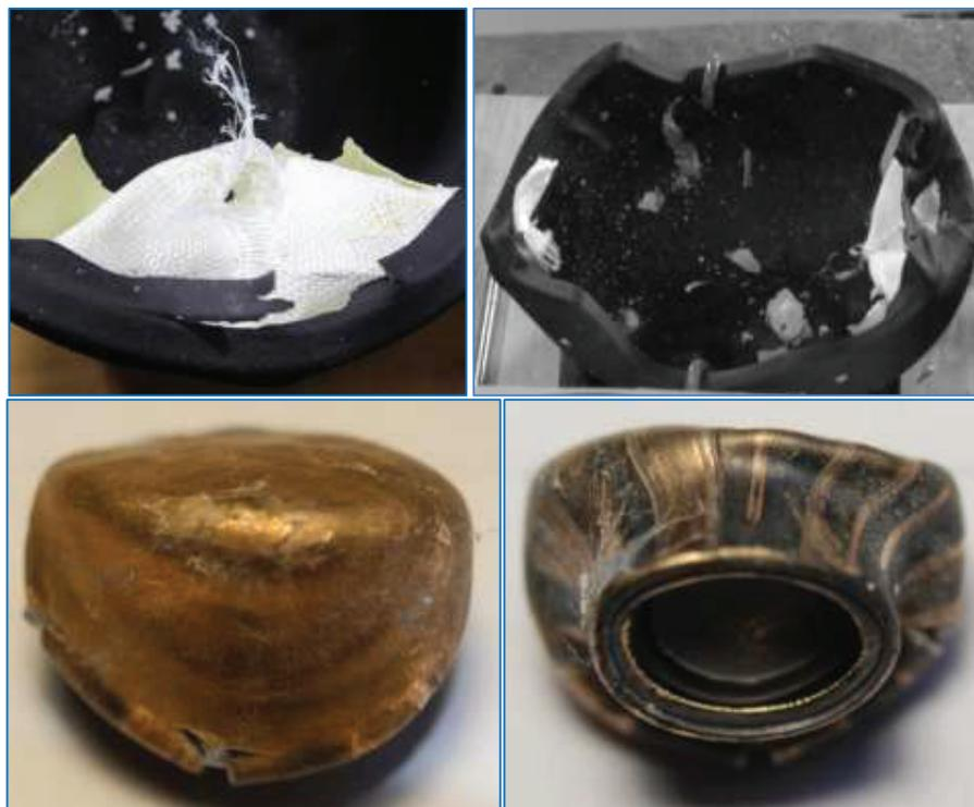
**Figure 8.** Shot 2 on UHMWPE helmet PE2: permanent deformation (top left); high-speed still of temporary deformation (top right); recovered bullet (bottom)
