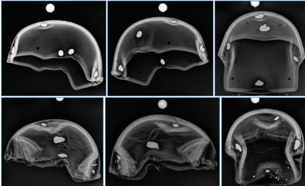
**Figure 6.** X-Rays of Para-Aramid Helmet PA1 (upper) and UHMWPE Helmet PE1 (lower) – Post-Test
