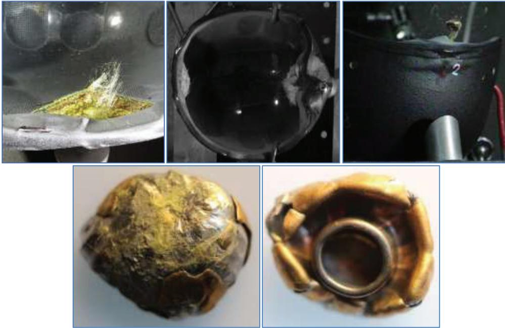
**Figure 10.** Shot 2 on para-aramid helmet PA3: permanent deformation (top left); high-speed still of temporary deformation (top right); recovered bullet (bottom)
