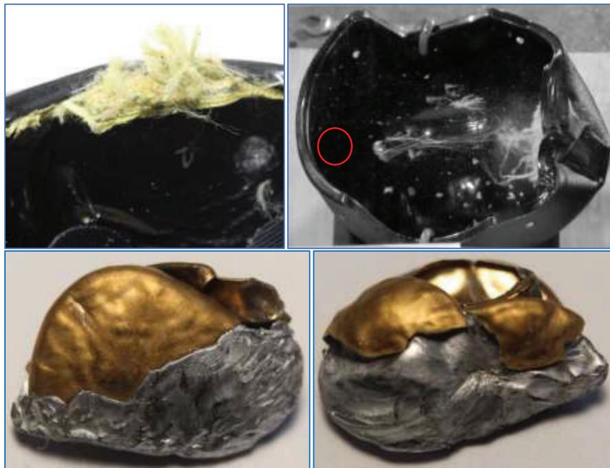
**Figure 7.** Shot 2 on para-aramid helmet PA2: permanent deformation (top left); high-speed still of temporary deformation (top right); recovered bullet (bottom)
