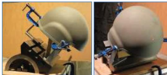
**Figure 2.** Helmet mounted to Test Rig in Typical Orientation
