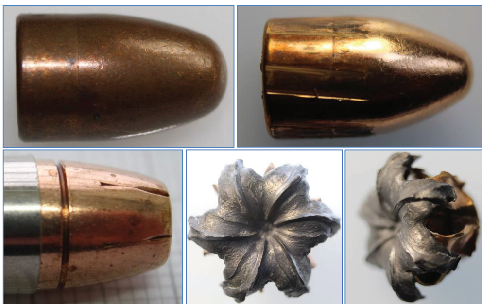
Figure 5. Pre-Fired (left) and Recovered 9 mm FMJ (upper) and 9 mm HP (lower)
