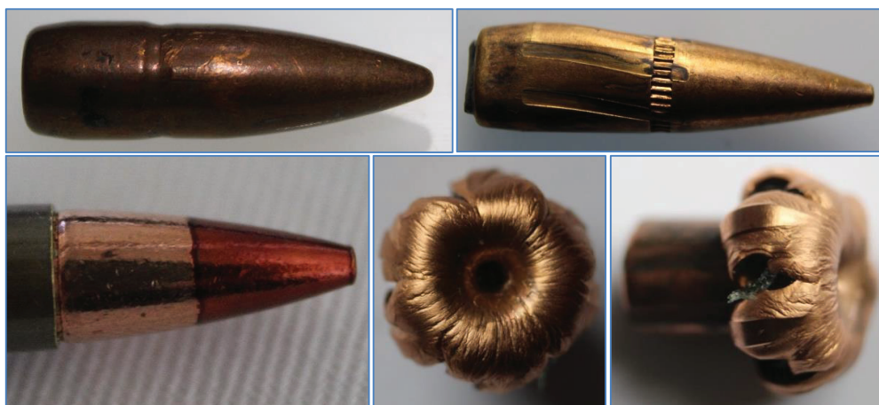
Figure 6. Pre-Fired (left) and Recovered 5.56 mm FMJ (upper) and 5.56 mm HP (lower)
