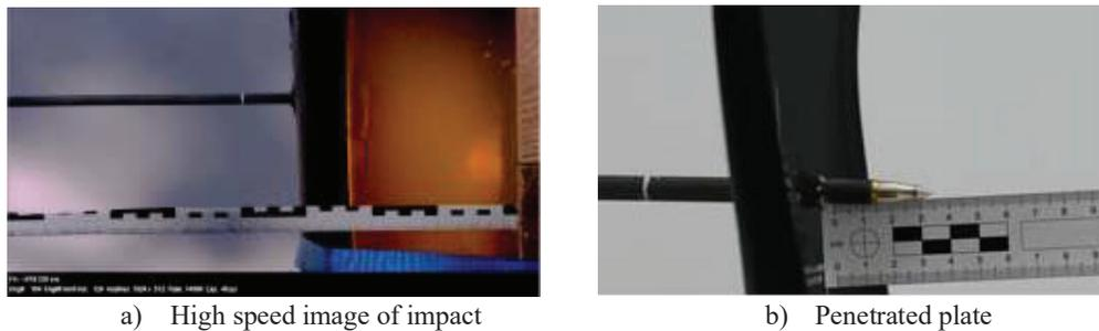
**Figure 13.** Bolt PEN I perforates ICW plate at 149 m/s
