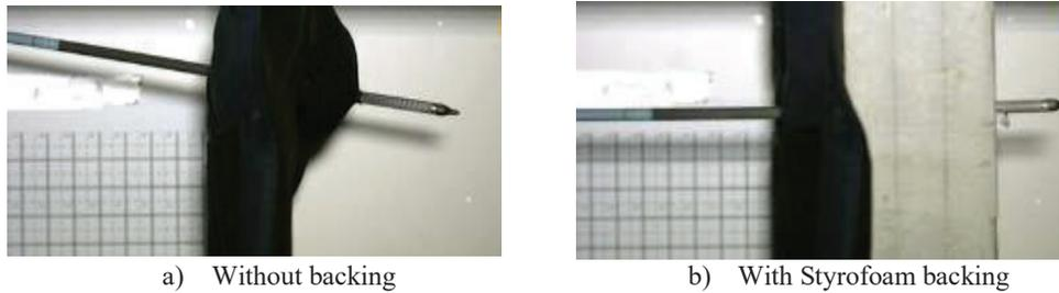
**Figure 1.** Arrow with penetration tip perforates soft body armour
