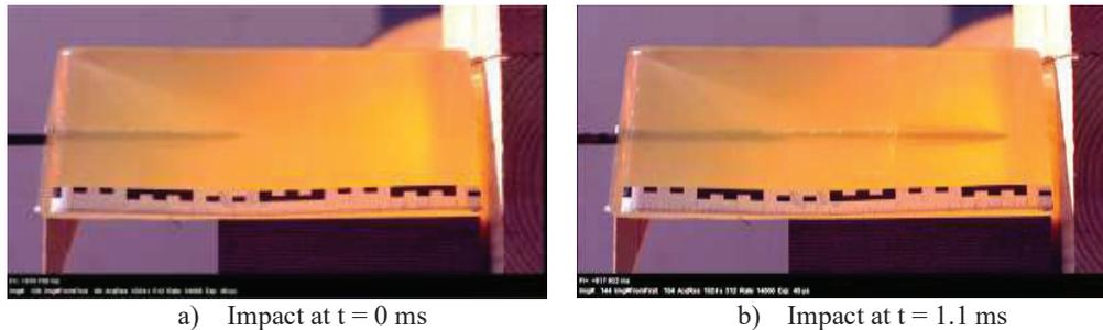
**Figure 17. Depth of penetration test in gelatine**
