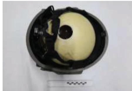
b) Head simulant inside the helmet
