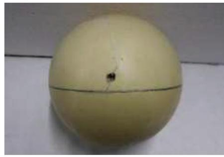
b) Head simulant damage signature
