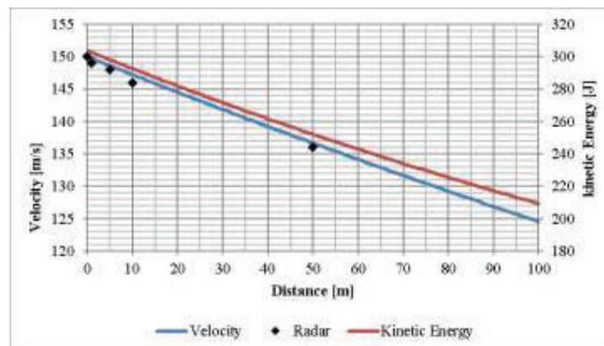
**Figure 5.** External ballistics of bolt (STANAG 2920 without error correction)
