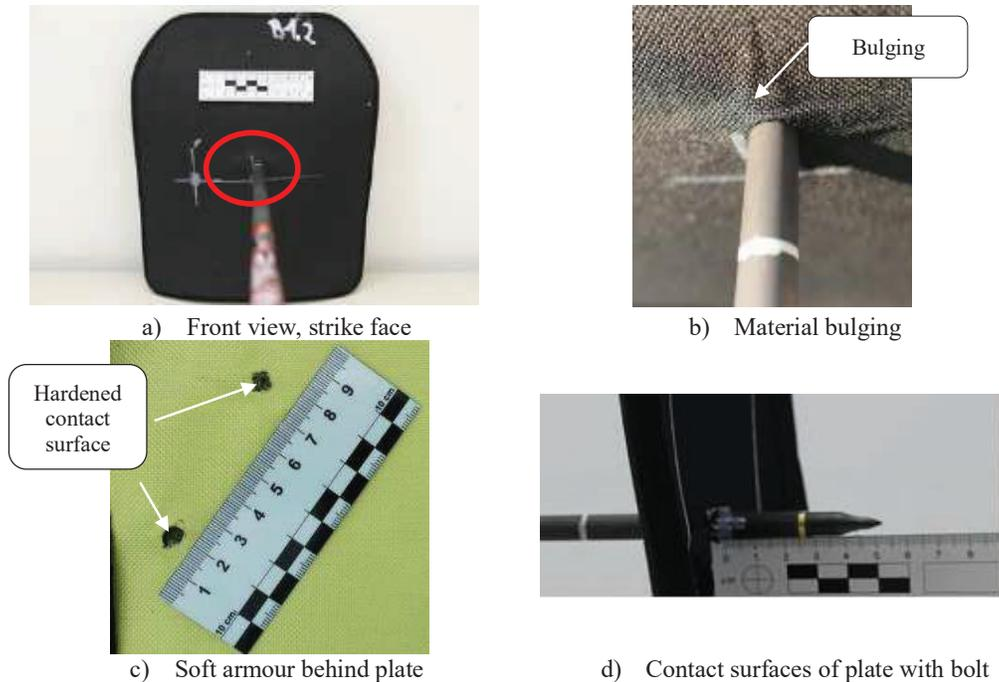
**Figure 12.** Damage signature on hard ballistic body armour SK2
