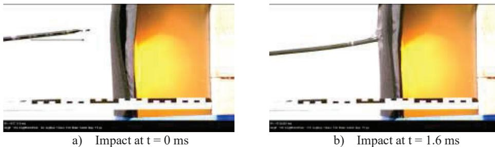
Figure 10. Bolt PEN II penetrates SK2 body armour at impact with yaw
