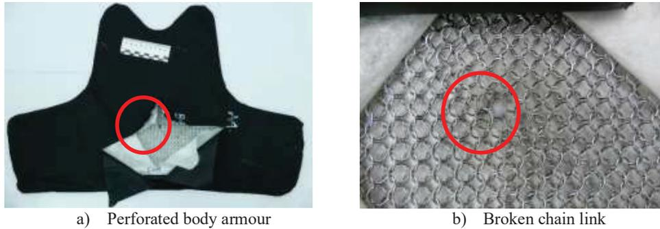
Figure 9. Damage of the chainmail upon perforation of a bolt with PEN II at 146 m/s
