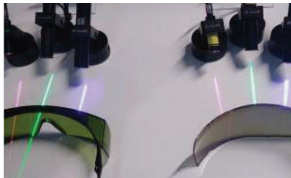
**Figure 2.** Experimental evidence of successful RGB blocking by the blank (right, absorption filter) as compared to conventional laser protection glasses for usage in a laboratory environment (left).
