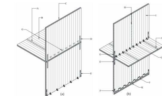
Figure 1. Walls and floors in CLT structures: (a) single-panel and (b) multi-panel [4]
