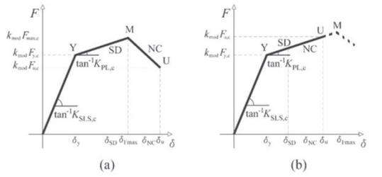
Figure 3. Derivation of the trilinear (a) and bilinear (b) load-deformation mean curve of dissipative zones in timber structures made with metal plate connectors and 3D-connectors [4]
