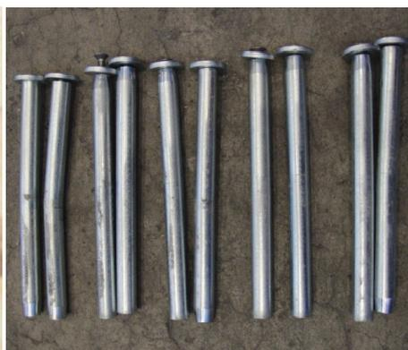
Figure 18. Dowels state of type B testing.
