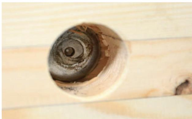
Figure 17. Embedding of timber at connection with the dowel.
