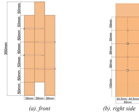
Figure 2. Specimens size and shape
