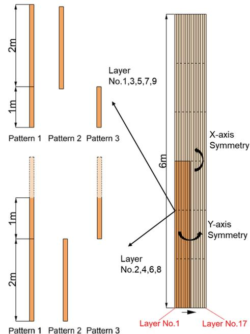
Figure 6. Lumber arrangement method
