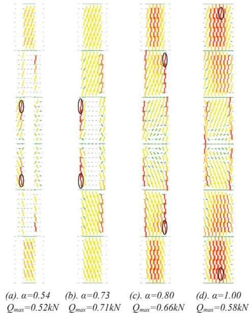
Figure 11. Shear force distribution
