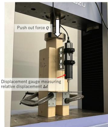
Figure 3. Test setup and measuring method
