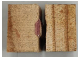
Figure 6. Non-planar surface of failed specimen.
