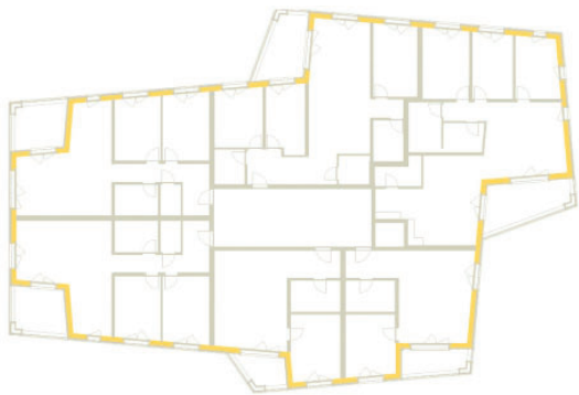
Figure 3. Floor plan from the first to the third floor along the main axes measuring approximately 36 x 26 metres. Source: Renggli AG
