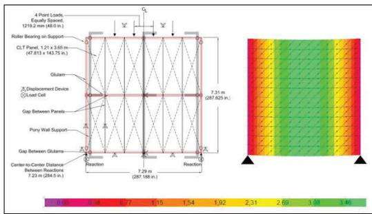
Figure 5. Scheme of CLT diaphragm carried out by Line et al [21] modeled with Veliz et al [18] methodology.
