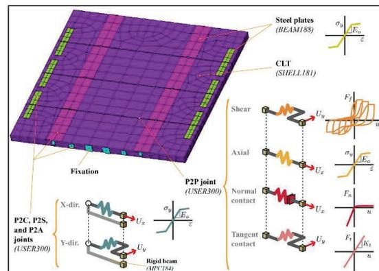
Figure 11. Non-linear detailed ASPID model depiction
