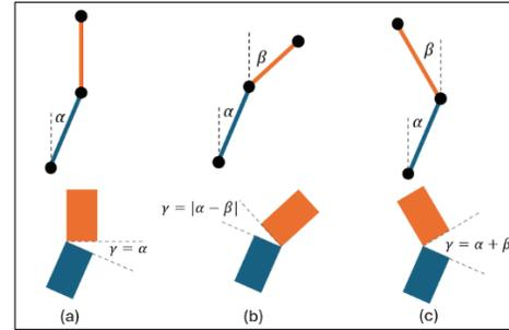
Figure 4. Different types of column relative rotations and their influence on splice deformation.
