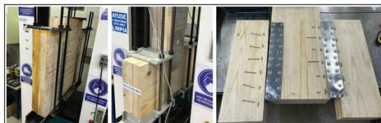
Figure 9. Testing of inter-panel and chord straps connectors.
