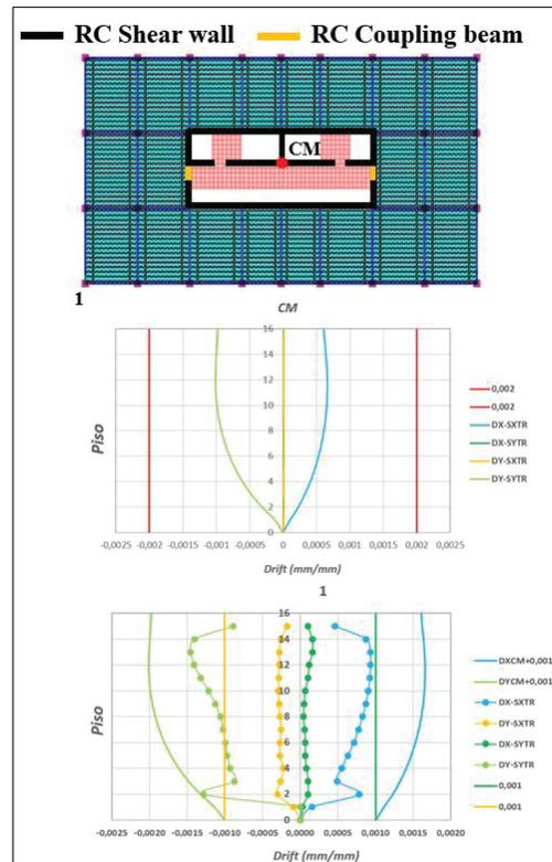
Figure 7. Torsional drifts for Office building (Fig. 1(a)).
