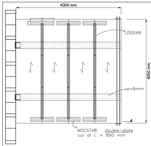
Figure 10. Full-scale diaphragm specimen testing setup.
