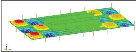
Figure 3. RFEM 6 modal analysis displacement contour results for the first vertical mode ( $f = 10.37$  Hz)
