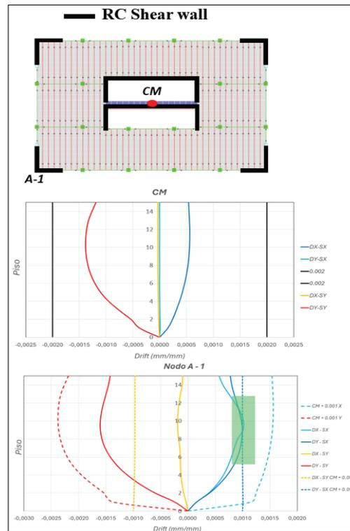
Figure 6. Torsional drifts of preliminary building (Fig. 2).
