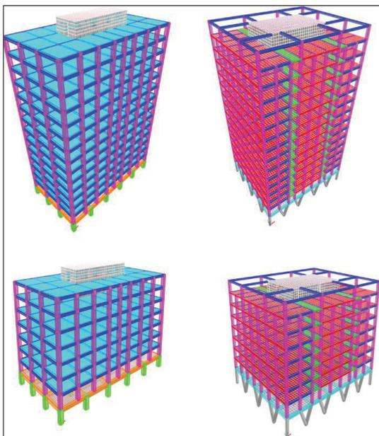
Figure 8. Isometric view of 8 and 15 story ETABS models of Office (left) and Residential (right) buildings.
