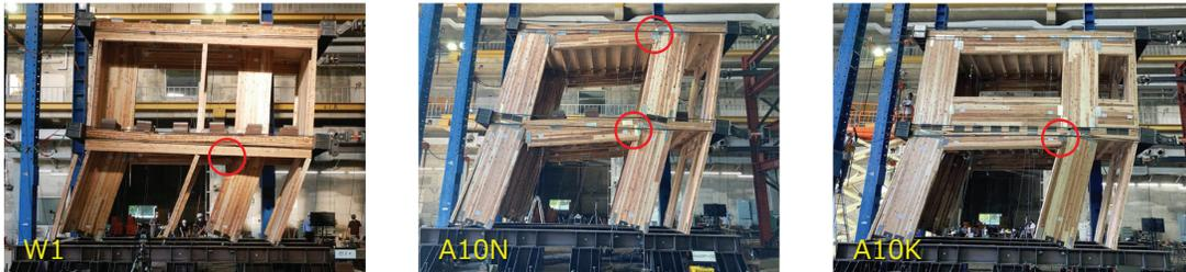
Figure 7. States of deformation near the provisional collapse limit
