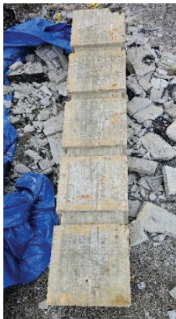
Figure 5. The glulam column recovered after the pilot fire test.
