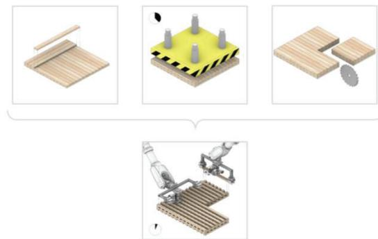
Figure 3: From a subtractive to an additive manufacturing approach.
