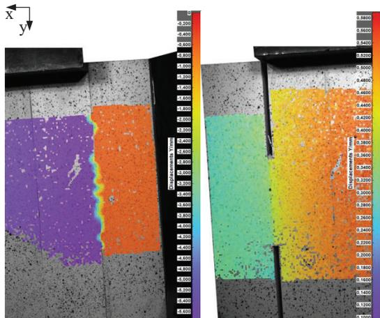
Figure 6: Digital image recording displacements  $y$  [mm] in test configuration 0° for a 16 mm dowel (left) and for beech nail Adhesive 1 (right) with pressure close to the failure point
