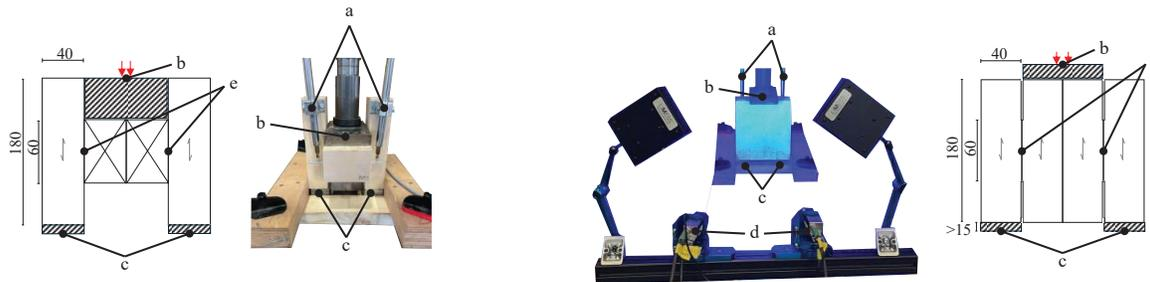
Figure 4: Test specimens and experimental setup 90° (left) and 0° (right) with (a) displacement transducers, (b) load point, (c) force measuring device, (d) digital image correlation system, (e) investigated shear plane.
