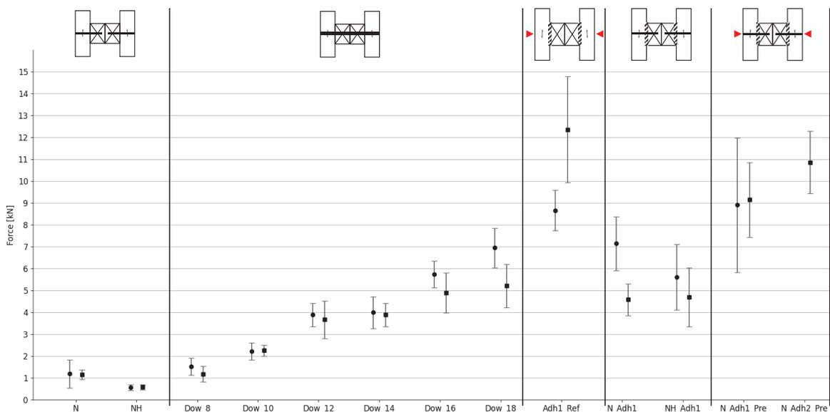
Figure 5: Mean maximum shear load and standard deviation per side in [kN] for configuration 0° (●) and 90° (■)
