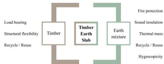
Figure 1: Combined characteristics of a timber earth slab
