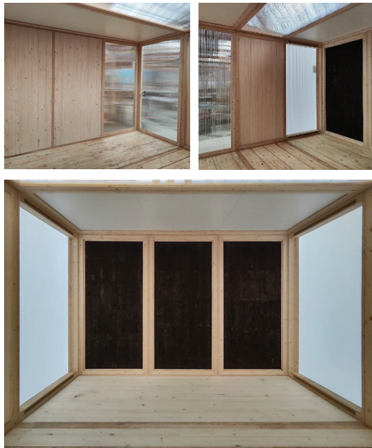
Figure 138. Different layers tested in prototypes built in DISPO hall providing visual, transparency and sound-insulation properties.
