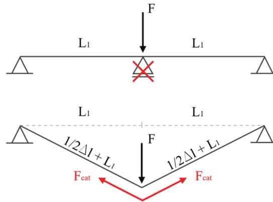
Figure 1. Catenary system over two floor spans
