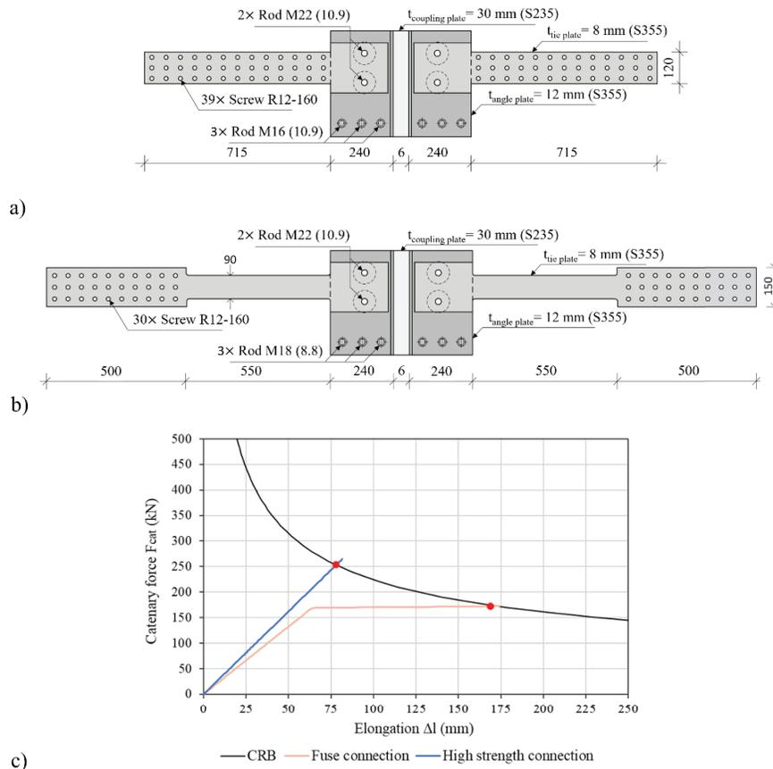
Figure 5. Optimized inter-modular connection design based on a) Method 1: increasing axial resistance and, b) Method 2: increasing ductility.
