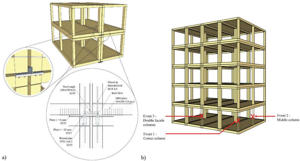
Figure 2. Case study project description, a) module and inter-modular connection design, b) column removal scenarios.
