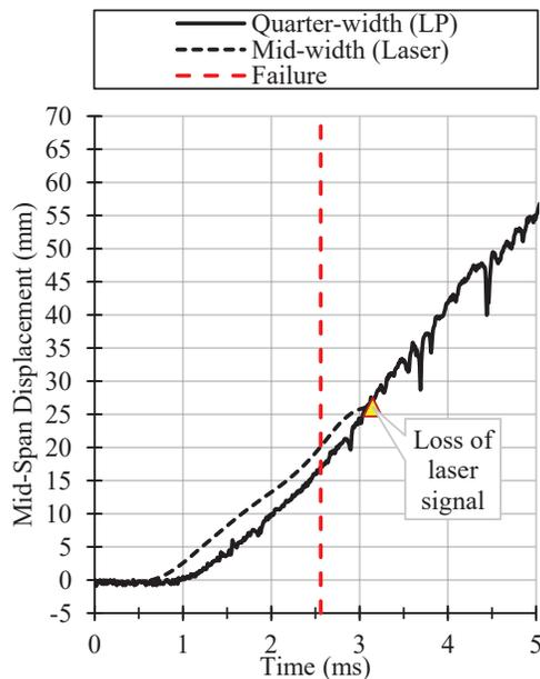
Figure 4: Representative near-field blast displacement-time history
