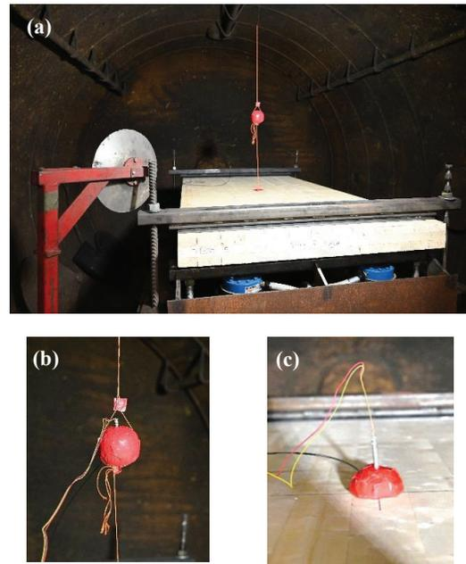
Figure 2: (a) Experimental test setups (b) near-field C4 charge (c) C4 contact charge
