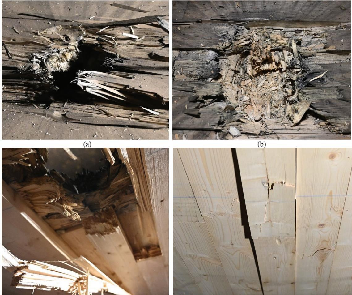
Figure 9: 200g C4 contact charge on (a) 3-ply panel (full breach) (b) 7-ply panel (no breach and localized cracking and FJ failure)
