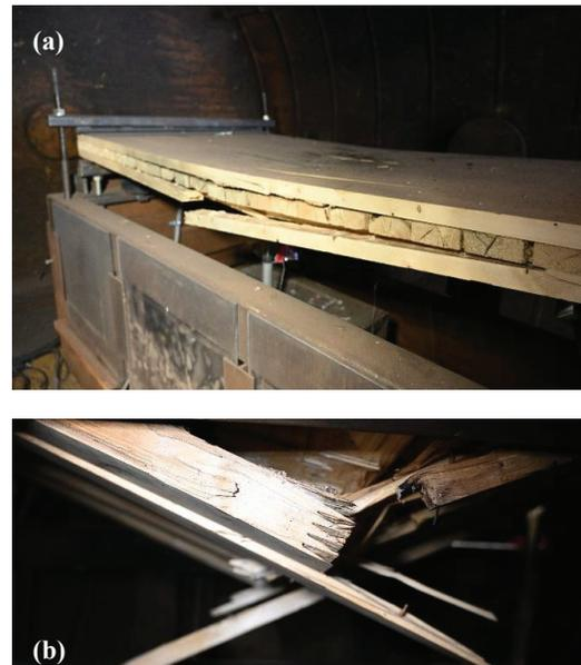
Figure 5: Representative (a) flexural failure (3-ply specimen) (b) finger joint failure
