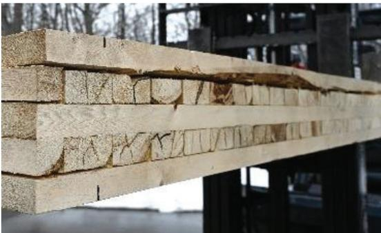
Figure 7: Rolling shear failure in 5-ply specimen
