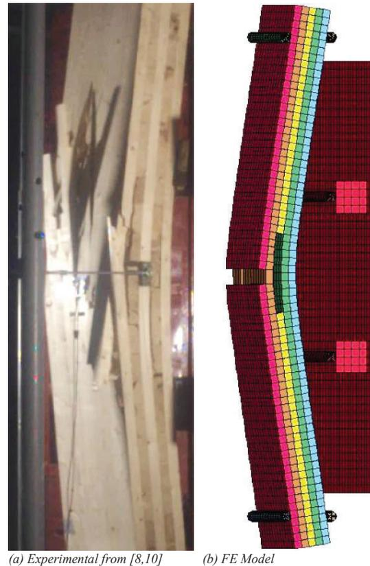
Figure 4. Representative results for CLT (CLT1.1)
