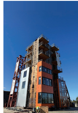
NHERI Converging Design 6-story Building Specimen
