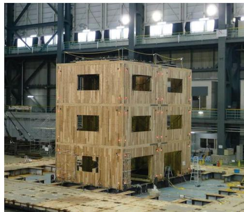
Figure 9 Three story specimen with wide panels
