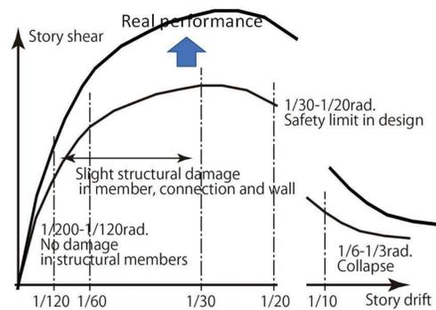
Figure 2 Limit state in design and real performance
