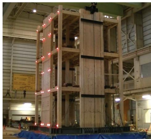
Figure 12 Rocking shear wall system
