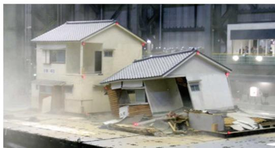
Figure 7 Existing house with/without reinforcement
