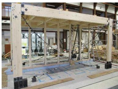
Figure 5 Post and beam construction with damper
