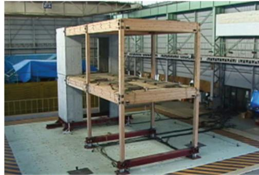
Figure 8 Post and beam construction with R/C corer
