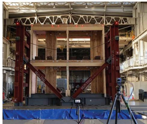
Figure 11 Two-story CLT construction to evaluate collapse limit
