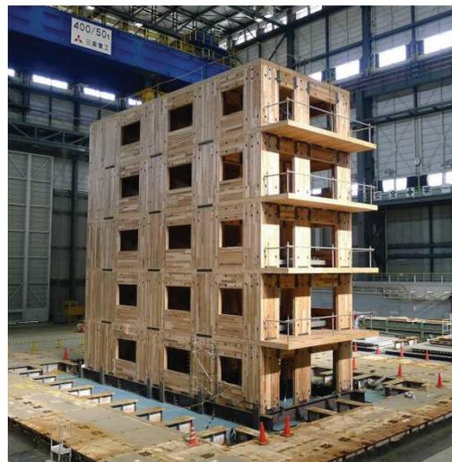
Figure 10 Five story specimen with narrow panel
