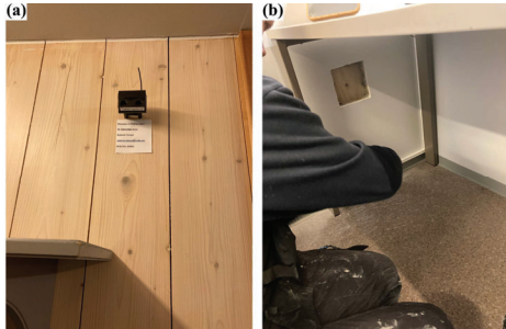
Figure 2. a) A typical sensor monitoring the MC of wood, and (b) plaster removal at some locations.
