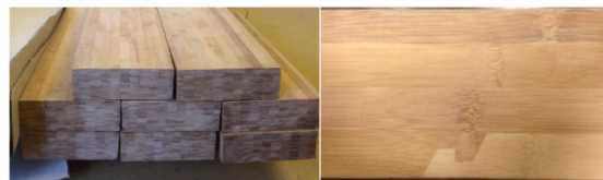
Figure 1. Cross section of laminated bamboo beam (left) and face showing a bamboo strip with hook joint (right).
