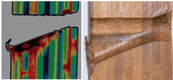
Figure 10). Density variation over a cross section around a deformed dowel. The densification on the lower left side and upper right side is where the dowel crushes the bamboo fibres.
