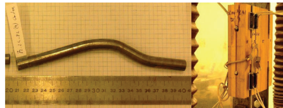
Figure 8. Non-symmetrically failed dowel from a double slotted-in steel plate connection.
