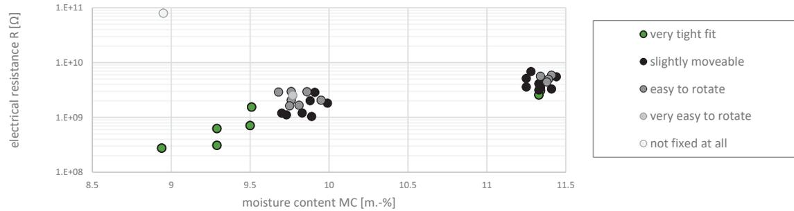
Figure 10: Results, as shown in Figure, sorted by the electrodes' manually determined tightness of fit at 23 °C
