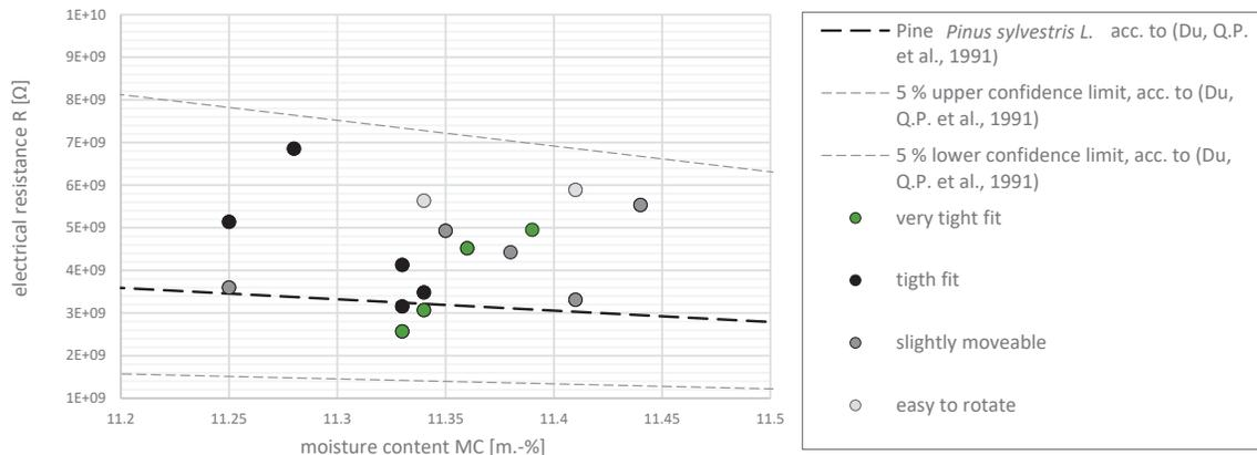
Figure 3: Tightness of fit for electrodes in radiata pine after preconditioning at  $23\pm 0.5\text{ }^{\circ}\text{C} / 57\pm 2\text{ \%RH}$  for >65 days; juxtaposed to the calibration curve for Scots pine by (Du et al., 1991).
