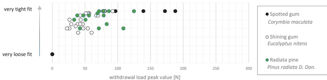
Figure 5: Results of first measurement series showing a correlation between withdrawal peak load capacity [N] and manually estimated movability of electrodes in three different subtropical wood species; measurements at mass constancy, after steady pre-conditioning at  $23 \pm 0.5\text{ }^\circ\text{C} / 57 \pm 2\text{ \%RH}$  for 65 days
