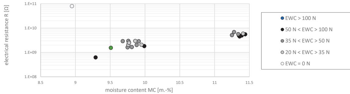
Figure 9: Selection of measurement results shown in Figure, sorted by their electrode withdrawal peak load capacity  $EWC$  [ $N$ ] at 23 °C
