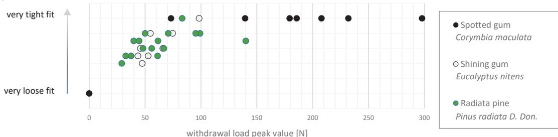
Figure 6: Results of second measurement series showing a correlation between withdrawal peak load capacity [N] and manually estimated movability of electrodes in three different subtropical wood species; measurements after climate step change to  $35 \pm 1\text{ }^\circ\text{C} / 36 \pm 5\text{ \%RH}$  for 45 hours, possibly with moisture gradients in the specimens
