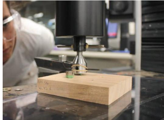
Figure 2: Electrode withdrawal testing with the Instron UTM on a sample from shining gum
