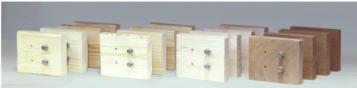
Figure 3: Selection of four charges of specimens for electrical resistance measurements with pin-type electrodes for wood moisture content determination.
