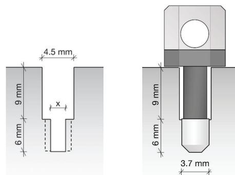
Figure 1: Cross section of predrilled holes and final fit of 15 mm rammed-in electrode
