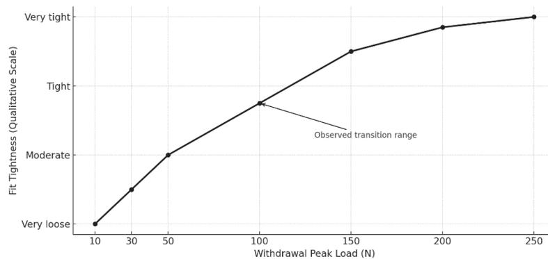
Figure 7. Schematic Relationship Between Withdrawal Load and Electrode Fit
