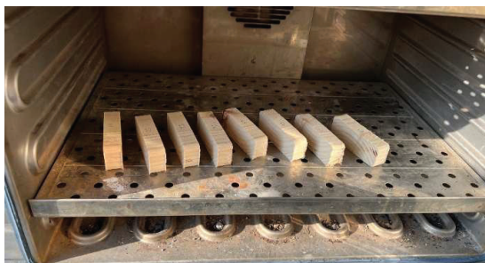
Figure 1. Samples of C16 timber in oven for the determination of moisture content
