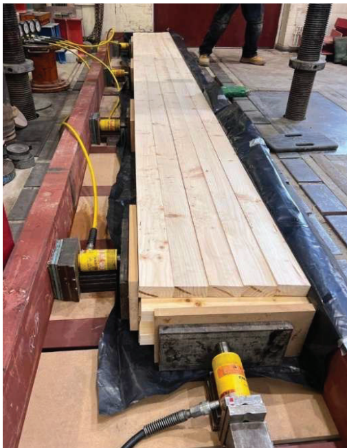
Figure 2. Manufacture of CLT panel involving the lateral pressure application
