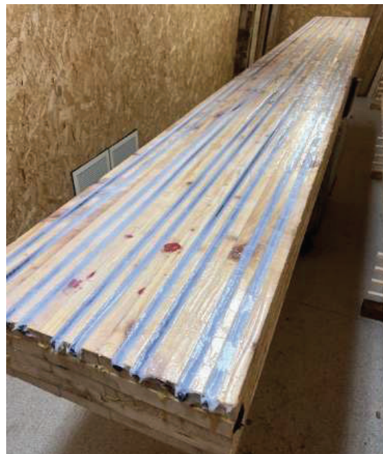
Figure 4. CLT panel with additional rebar reinforcement
