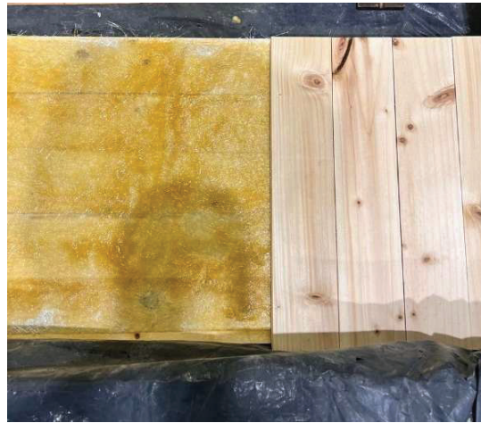
Figure 3. Glass fibre matting applied between the layers of timber, bonded using one component adhesive
