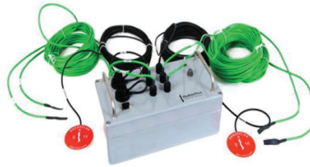
Figure 3 Heat Flow Method (HFM - https://www.hukseflux.com/products/heat-flux-sensors/heat-flux-meters/hfp01-heat-flux-sensor ) and Temperature Based Method (TBM) instruments setup
