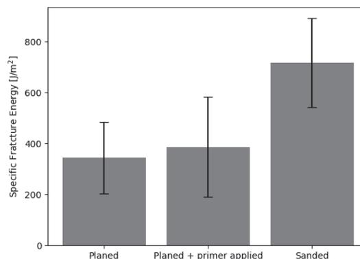
Figure 6: Specific fracture energy results of bonded beech wood with different surface preparation methods prior adhesive bonding.
