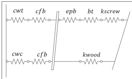
Figure 4. Scheme of the deformability components of the steel-timber joint
