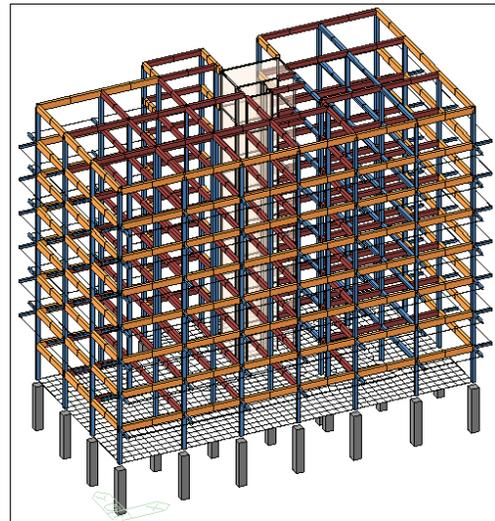
Figure 2. Numerical model of the eight-story frame building without infills (M1 and M2 models)
