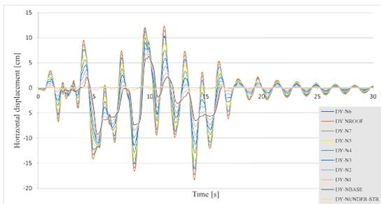
Figure 9. Horizontal displacements-time diagram for all the building levels (M4 model)
