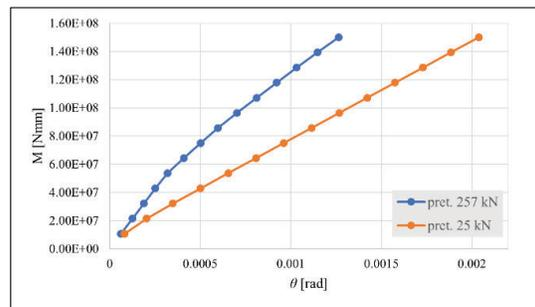
Figure 6. Moment-rotation curve of the steel part of the joint for pretensioned bolts (blue) and non-pretensioned bolts (orange)
