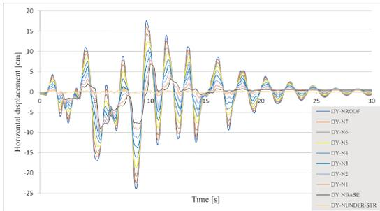
Figure 8. Horizontal displacements-time diagram for all the building levels (M1 model)
