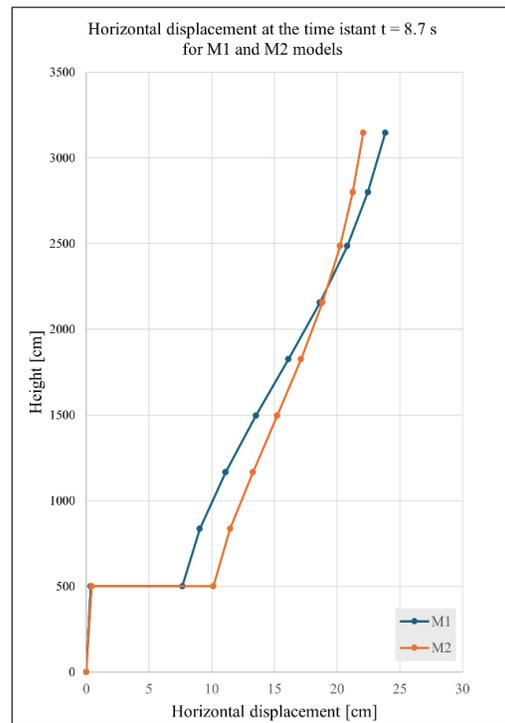
Figure 10. Horizontal displacements at the time instant  $t = 8.7$  s for M1 (bare and semi-rigid node model) and M2 (bare and rigid node model) models
