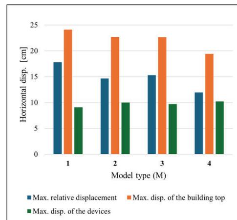
Figure 7. Comparison of horizontal displacements from numerical analysis between model configurations
