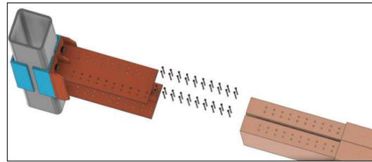
Figure 1. Steel column to timber beam joint technology
