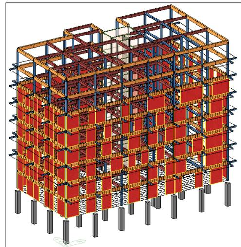
Figure 3. Numerical model of the eight-story frame building with infills (M3 and M4 models)
