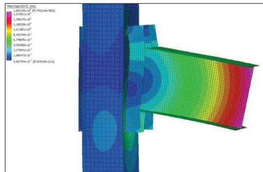
Figure 5. FE model of the steel part of the beam-to-column joint
