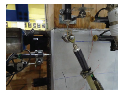
Compression side at column-to-joint connection at 1/100rad.
