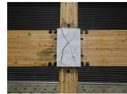
Specimen after the test No. 2 Column Bending Failure
