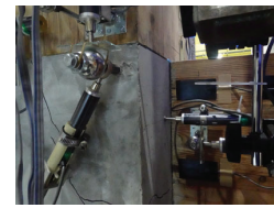
Tensioned side at column-to-joint connection at 1/100rad.
