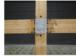
Specimen after the test No. 1 Beam Bending Failure
