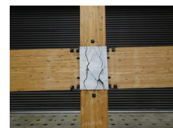
Specimen after the test No. 3 Panel Shear Failure
