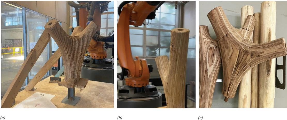
Figure 10. The robotic milling of the node blank showing (a) the first rough milling pass of vertical contouring, (b) the final cross lacing pass to achieve a smooth finish, and (c) the completed and sanded node. Also visible are the dowel pockets and the inserted dowel in the bottom of the primary node arm.
