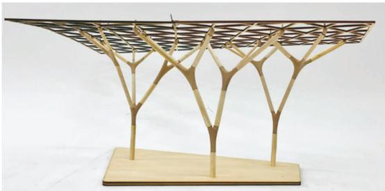
Figure 1. A model of the pavilion, made of 3D printed nodes, laser cut canopy and dowel members.
