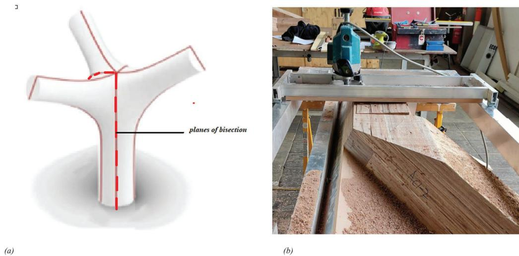
Figure 8. (a) The planes of bisection on the primary branch of the node arm. (b) Gantry and router showing planing of one of the planes of bisection.
