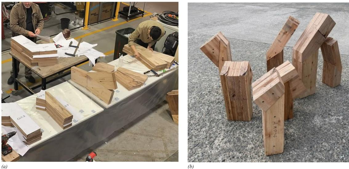
Figure 7. (a) Assembly, glueing and clamping of the mitred LVL lamellas. (b) The completed custom profiled laminated billets.
