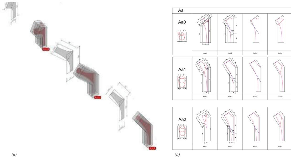
Figure 6. (a) The three node arm geometries making up a node, shown as side profiles and 3-dimensional views with the lamellas required to enable construction of a custom profiled billet. (b) Each node arm billet, shown in top view on the left, and side view on the right, showing the alternate mitring patterns of the LVL lamination.
