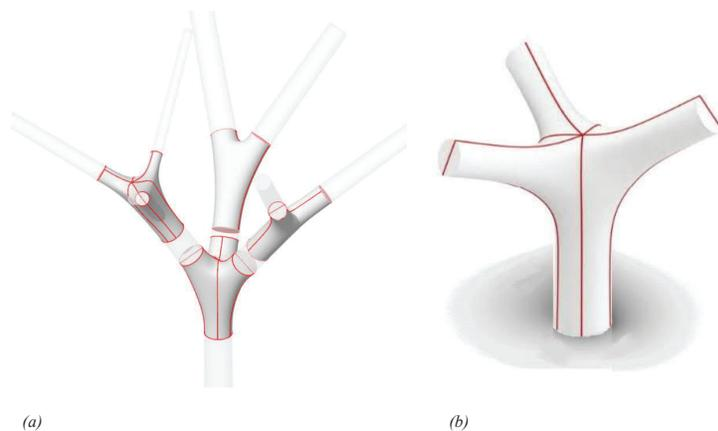
Figure 3. (a) A cluster of 2-way coplanar and 3-way non-coplanar nodes and their intersection with roundwood branch members. (b) An isolated example of a 3-way node. Note the red lines represent the planes of bisection.
