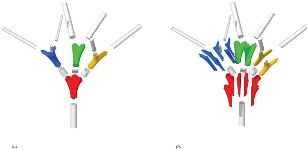
Figure 4. (a) The branches of the cluster shown in Figure 3, with nodes separated from adjacent roundwood members. (b) Now shown bisected by the planes that are common to both the primary (lowermost) node arms, and each of the departing (uppermost) node arms. Note the relative simplicity of the 2-way co-planer node being bisected just once, resulting in two parts, versus the 3-way node being bisected three times, resulting in six parts.
