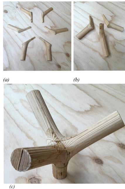
Figure 5. Prototyping of a non-coplanar node at 1:5 scale, showing (a) the 6 individual node parts machined prior to assembly, (b) assembly of the 3 upper branches about their individual common planes, and (c) assembly of the complete node with the all branches assembled about the single common axis of the primary lower branch.
