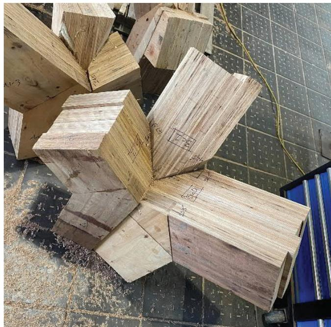
Figure 9. A glued node blank, ready for final machining. Three custom laminated node arm billets are glued together about the central axis of the primary node arm.
