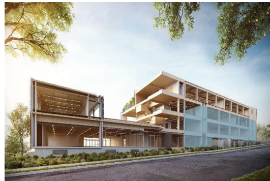
Figure 10. Perspective section rendering of OLA Stage 2, existing concrete frame highlighted on right.
