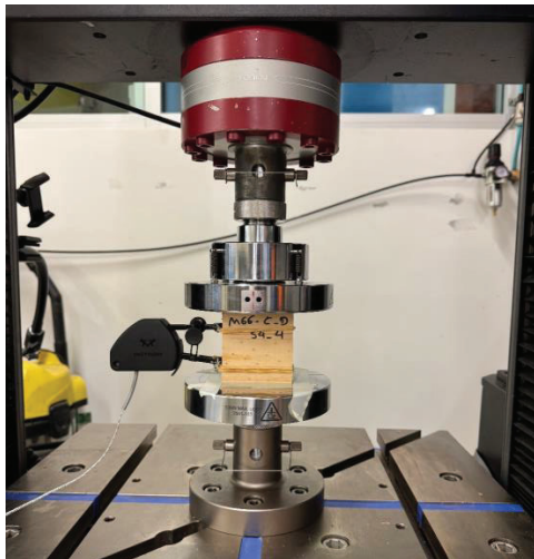
Figure 4. Setup for perpendicular-to-grain compression tests
