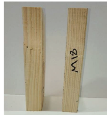
Figure 8. Failure modes of representative samples tested parallel-to-grain (a) front view, and (b) side view
