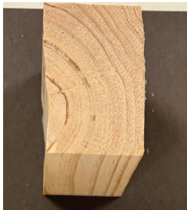
Figure 11. Failure mode of representative samples tested perpendicular-to-grain (a) front view, and (b) side view
