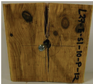
Figure 7. Front view of representative samples tested parallel-to-grain experiencing (a) no load drop, and (b) a load drop
