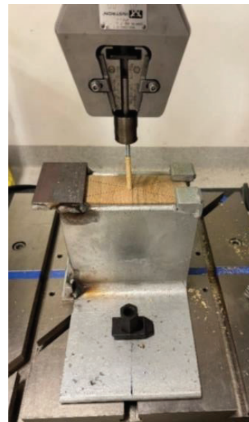
Figure 2. Withdrawal pull-out test set up
