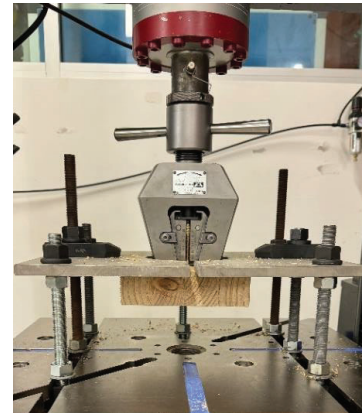
Figure 4. Withdrawal pull-through test set up
