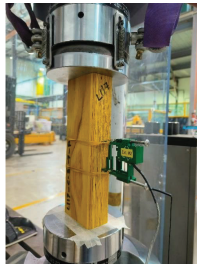
Figure 2. Compression test setup
